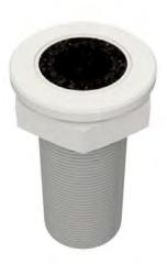
Benarx<sup>®</sup> Fire Drain Plug is an effective and automatic drainage system. It functions as ventilation (air-flow) with dissipate heat/gas build-up away whilst maintaining fire integrity during the fire as it will seal off the hole by swelling.
