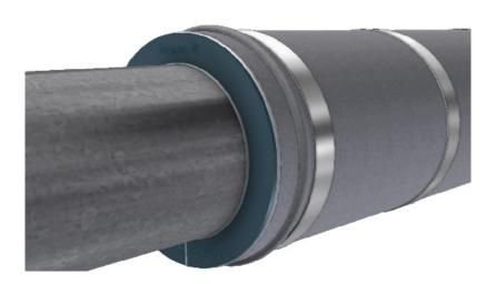
End termination of pipe insulation is a critical point of water proofing the pipe insulation material. Preparing end termination of traditional metal insulation cladding may be challenging to achieve with water ingress as a result. Water under the insulation and potential damages to pipe coating due to sharp metal edges is major risk factor resulting in development of CUI.
